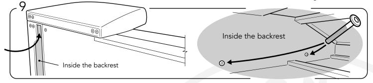
Close the chaise, turn it to the side and fix the armrest from inside the backrest with two M6 x 55 bolts.
